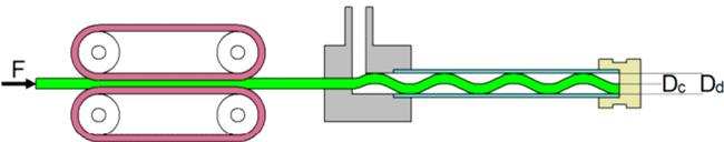
**Figure 7. Buckling of cable in duct**
