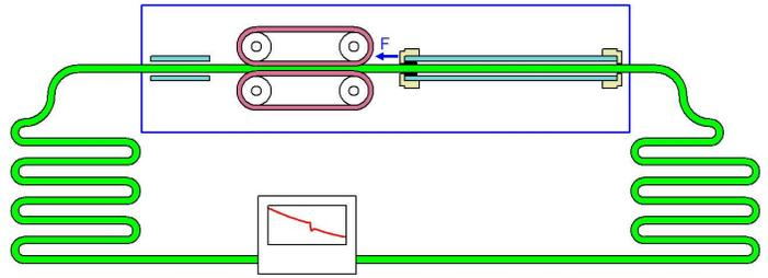
**Figure 8. Example of factory test under pulling force**
