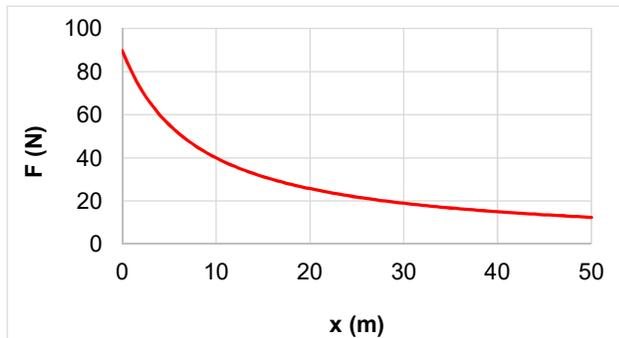
**Figure 10. Pushing force reduction for a 6.3 mm cable in a 50/40.8 mm HDPE duct**
