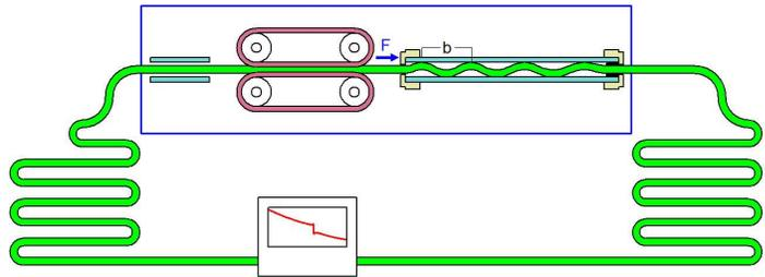
**Figure 9. Example of factory test under pushing force**
