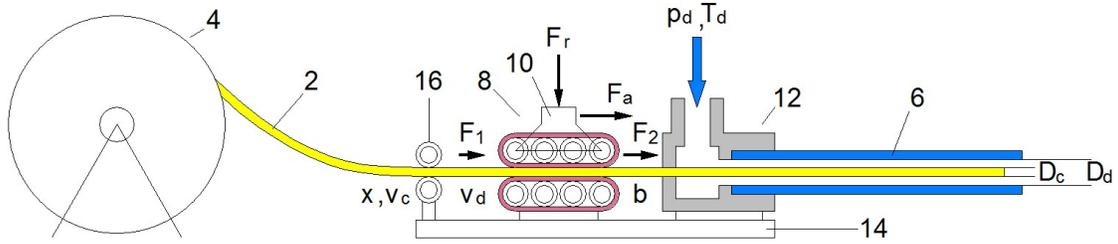
Figure 2. Functional drawing of "intelligent" jetting device
